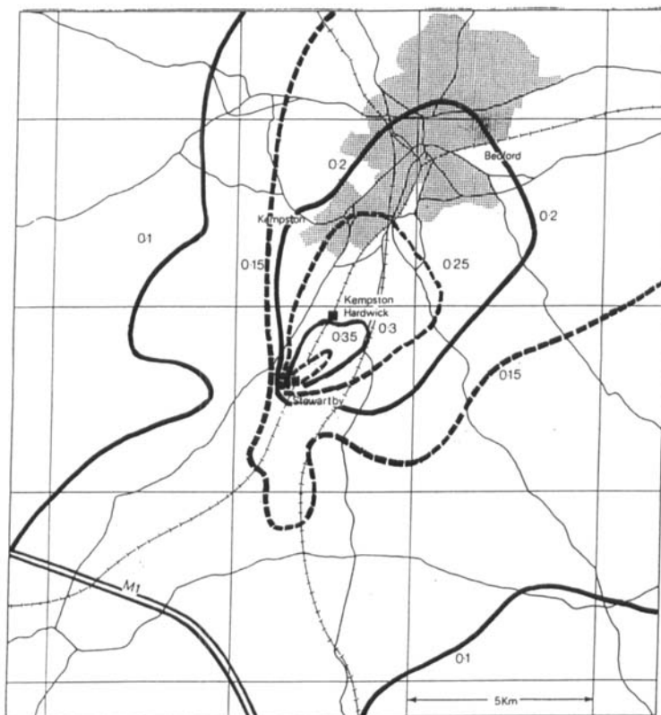
Figure 10 Contour map of airborne fluoride concentrations calculated by interpolation from sampling station data.
